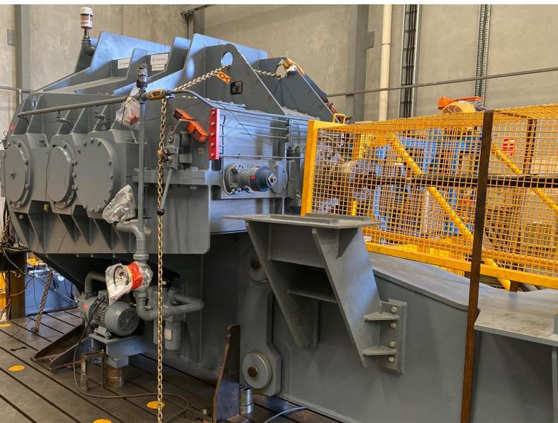
In addition to load testing gear units, WES will be able to load test the entire gearbox, motor and swing base assembly. This can be done as a shaft mounted assembly that closely replicates site mounting.
