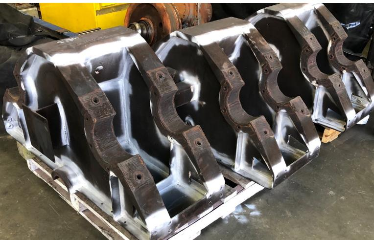
Our welded bronze pins are used in the 2 wheel bogie pin arrangement for Stackers and Reclaimers. We have specifically developed a process to achieve the required material fusion for this specific application.
