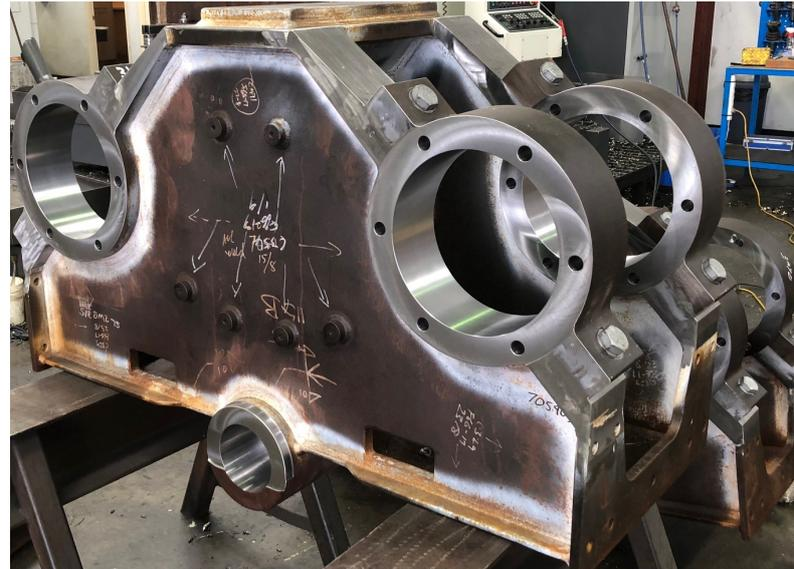
We also offer a vast range of refurbishment services. Pad & Bore welding on essential worn surfaces such as bearing journals is what we specialise in. In situations where important information for the required tolerances is missing, we have you covered through our Reverse Engineering Services. Our engineering department has the right methodologies to determine the missing sizes required for its specific application.
